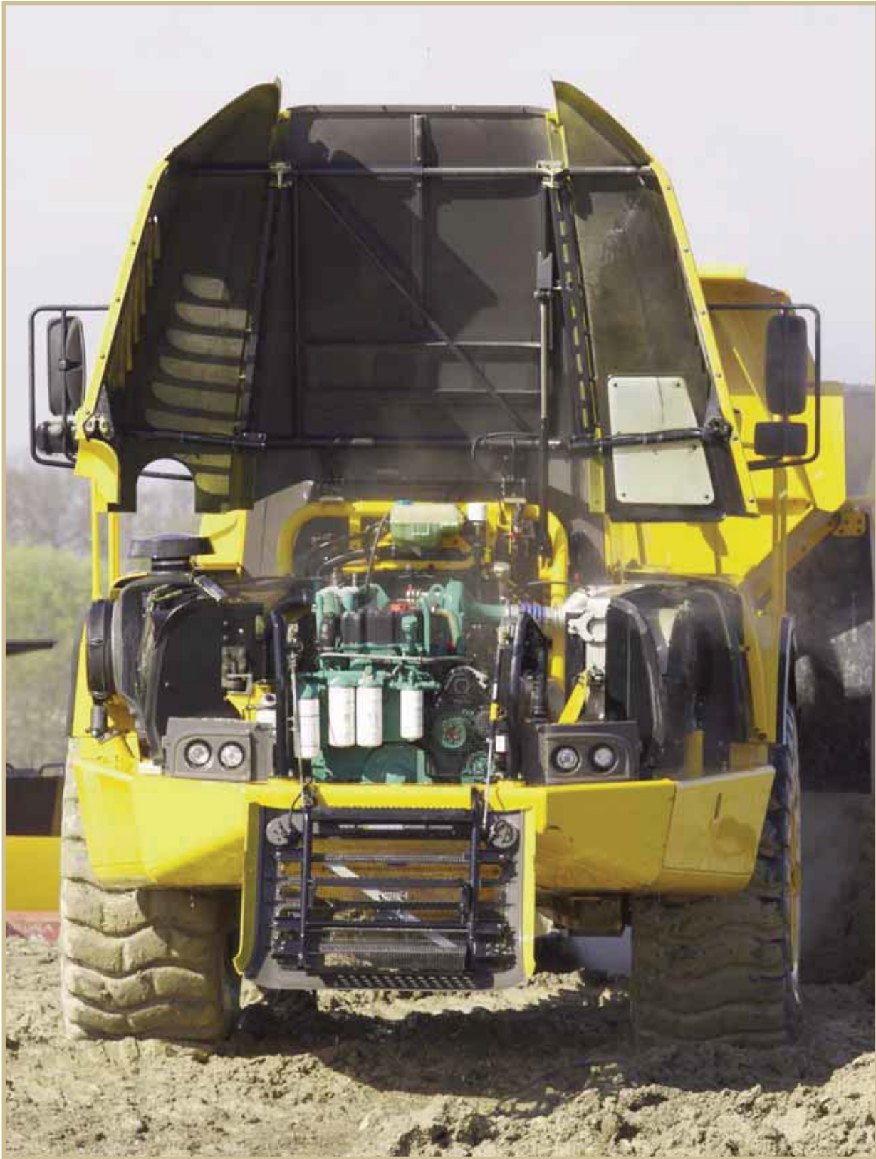
FIGURE 3—Heavy equipment like this dump truck depends on the high power delivered by a large diesel engine.
