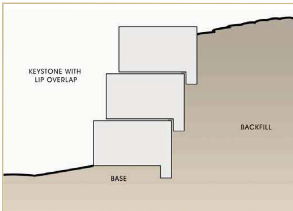
**FIGURE 12—Keystone is currently the material most commonly used for retaining walls.**
