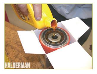
FIGURE 15—Filling the New Filter with New Engine Oil (Courtesy of James Halderman)
