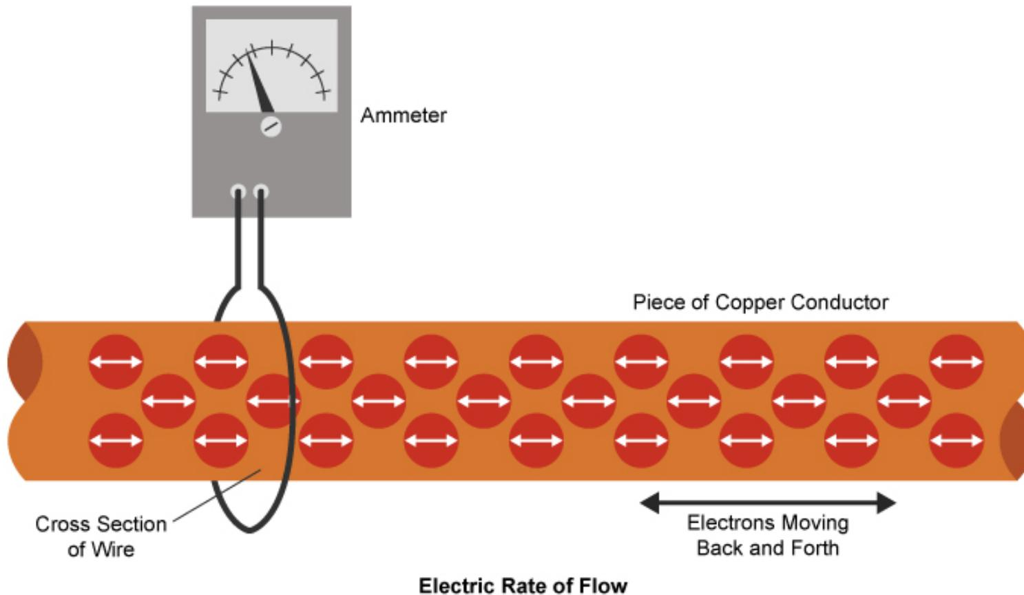
*The electrical current flow or amperage that can be measured with an ammeter is the rate of electron flow that passes through a cross section of wire.*
