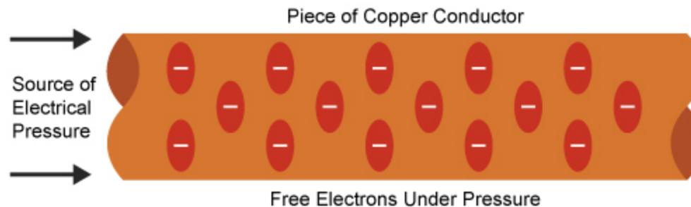
*When voltage (electrical pressure) is applied to a wire, the loose electrons are packed under pressure.*
