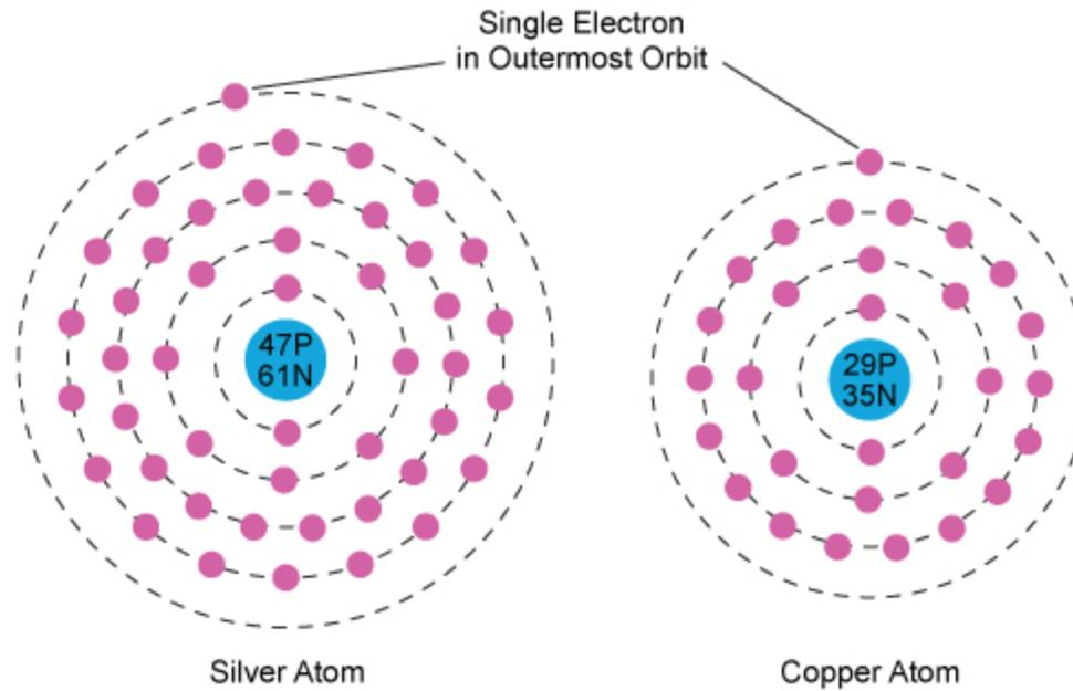
*Both silver and copper atoms have a free electron in their outermost orbits, and both are good electrical conductors. However, the free electron in the silver atom is farther away from the nucleus than the free electron in the copper atom. This means that the silver electron can be more easily dislodged from its orbit than the copper electron. Thus, silver is an even better electrical conductor than copper.*
