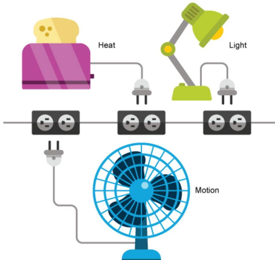
*Electrical energy is used to produce heat (in a toaster or space heater), to provide mechanical energy or motion (in fans and motors), and to provide light in a home.*
