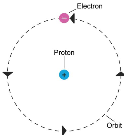
*A single atom of hydrogen contains one proton and one electron. The proton is represented by the circle with the plus sign (+) inside. The electron is represented by the circle with the minus sign (-) inside.*
