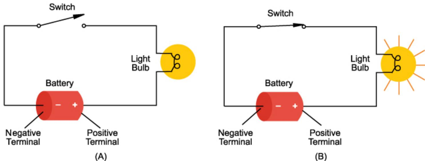
This figure illustrates a simple electrical circuit. In A, the switch is open, so electricity can't flow to the lightbulb. In B, the switch is closed, allowing electricity to reach the lightbulb.
