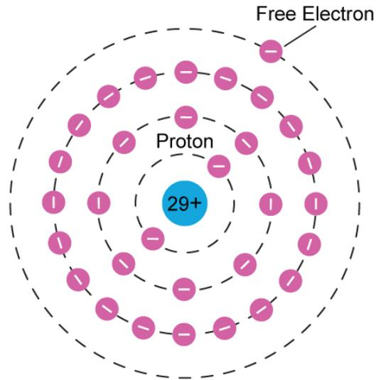
*A copper atom contains a single electron in its outermost orbit.
