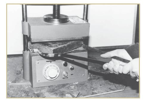
After removing the mold from the vulcanizer, place it in water to cool it. If you've molded an item with gemstones in place, splash water on it a little at a time. This gradual wetting will cool the piece at a slower rate. Some stones can't handle the shock of sudden cooling and may fracture if cooled too quickly.
