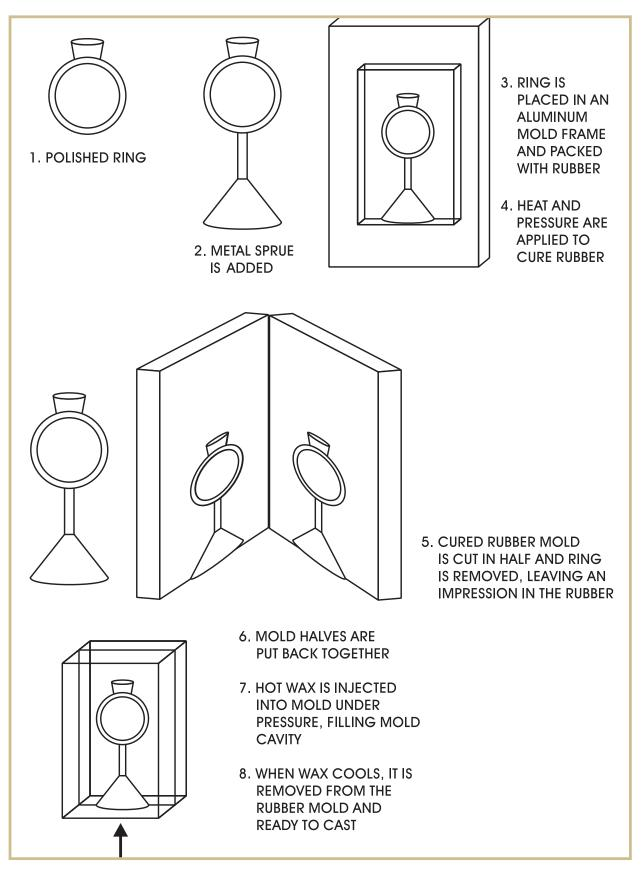
FIGURE 1—An Overview of the Moldig Process
