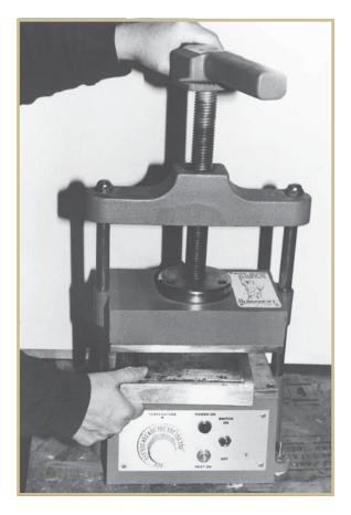
FIGURE 8—Removing Mold with Tongs
