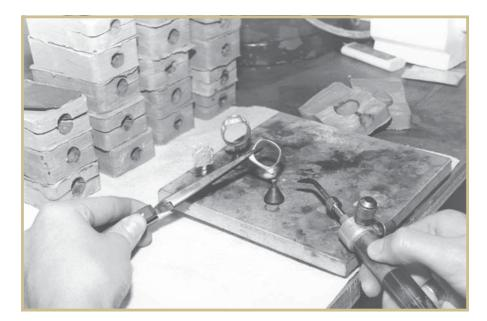
FIGURE 3—Soldering the Model to the Sprue Base
