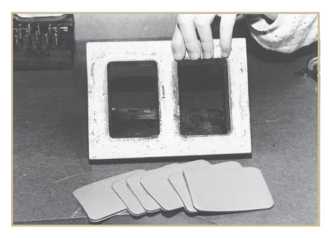
FIGURE 2—Sections of Precut Mold Rubber and a Mold Frame
